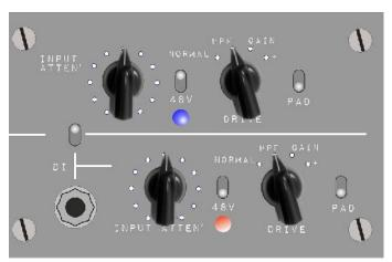
The input stage controls consist of: the DI switch (right/ side channel only); the input attenuation controls (both channels); the phantom power switches; the DRIVE rotary switches; and the pad toggle switches.
